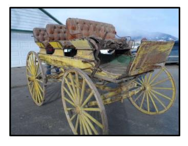
This wagon came to us in original condition retaining much of its original paint and pinstriping. All three bottom seat cushions were missing. The top, stanchions, and all mounting hardware were also missing.
