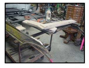
The original seat backs were cleaned and patched. New seat bottom cushions were built.
